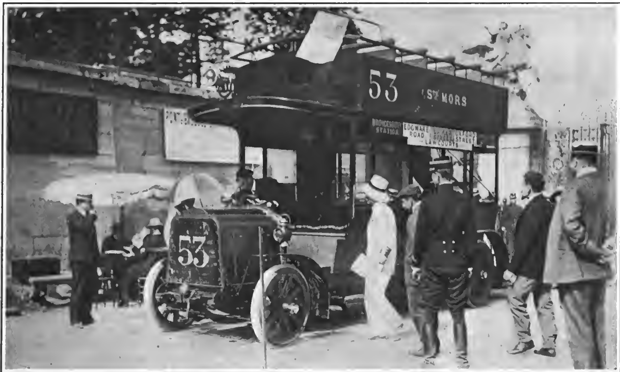
MORS OMNIBUS OF A TYPE BUILT FOR LONDON TRAFFIC WHICH WAS ENTERED IN THE FRENCH TRIALS.
